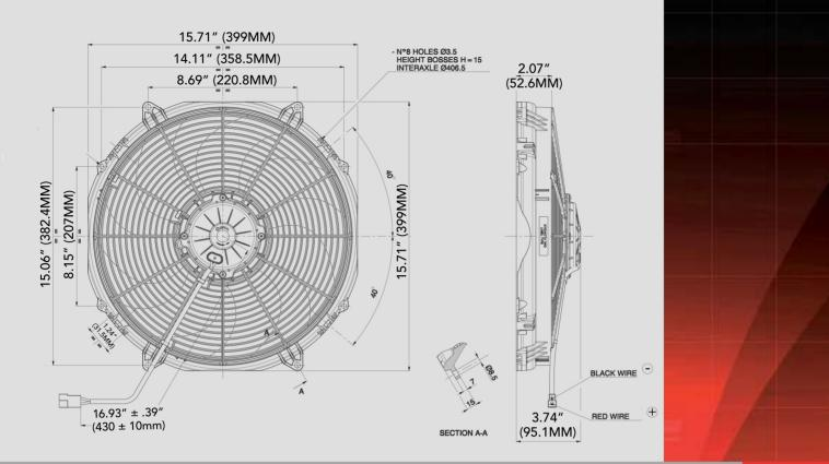
AMP connector Code 180908 AMP terminal Code 42098-2 Suggested mounting torque: 3(+1/-0) Nm with screw M5 Weight 2,84 Kg. approx.
