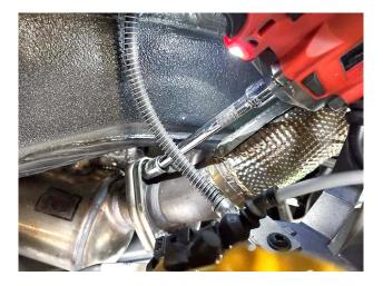
**Step 3:** In order to remove the over axle pipes without removing the rear exhaust, the studs must be removed from the over axle pipes. Use the double nut method to back out the factory studs and nuts.
