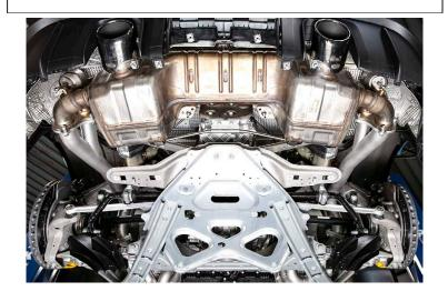
**Step 2:** Loosen header to over axle pipe hardware and remove nuts.
