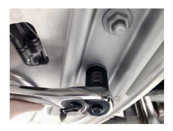
**Step 3C:** Each bolt can now be swung free to release band straps - remove them.
