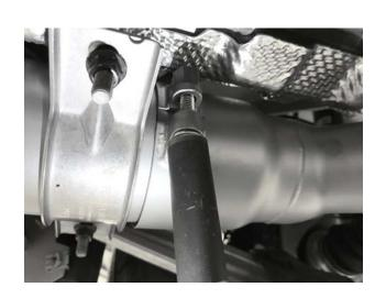
**Step 17:** Now that all downpipe clamps are in place and torqued down, replace and tighten chassic braces to 40-45 ftlbs .
