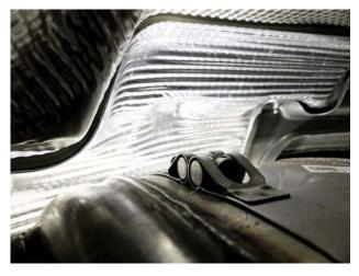
**Step 3A:** Locate the OEM band straps holding up the muffler on both the passenger and driver side.
