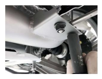
**Step 15:** Fully tighten OEM band strap onto the 90 degree downpipe section.
