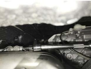
**Step 3B:** Loosen both driver and passenger straps but do not yet remove the 6mm allen bolt on them.
