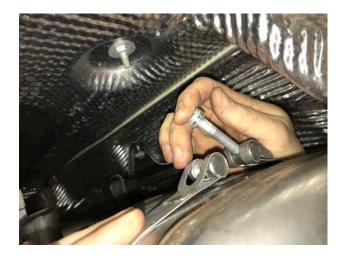
**Step 4:** The muffler is now being supported on these hangers. Lift the muffler and begin to pull towards the rear.
