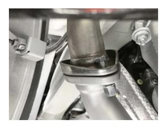
Correctly installed Sport Catalytic Converter downipe.
