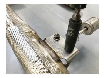
**Step 9:** Reinstall exhaust hanger on SOUL Y pipe. Snug the bolts but allow for slight movement for re installation.
