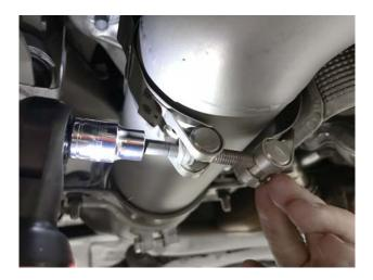
**Step 16:** Tighten both clamps holding downpipe sections together to 15-18 Ft LBS.
