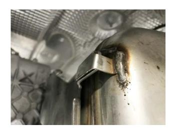
**Step 5:** The OEM muffler can now be removed from the vehicle. We recommend two sets of hands or the use of a jack to support the weight of the muffler as it is quite heavy.
