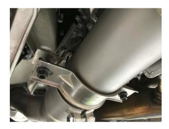
**Step 10:** Make sure the turbo and downpipe mating flanges are seated properly and install the OEM clamp on the cat section (with 90 degree bend section attached).
