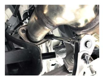
**Step 1:** Loosen and remove the 13mm flange nuts on both overaxle pipes on the factory exhaust.
