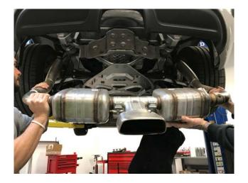
**Step 19:** Use included hardware to mate downpipe to rear exhaust.
