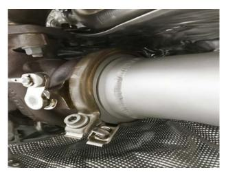
**Step 11:** Lift the new SOUL Y pipe section to the vehicle and start the exhaust hanger nuts to support the exhaust.
