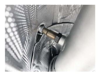
**Step 14:** Tighten exhaust hanger nuts to 12-15 Ft LBS.
