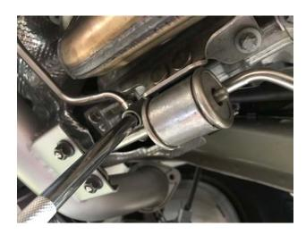
**Step 12:** Install exhaust bracket, torque to 15-18 Ft LBS.
