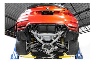
**Step 28:** Fully tighten the downpipe flange hardware at this time
