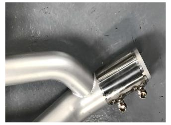
**Step 20:** Slide the previously installed sleeve clamps forward so they close the gap between the forward mid pipe and the mid pipe, do not fully tighten at this time.
