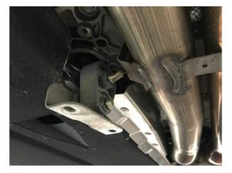
**Step 7:** With a friend or a jack, gently lower the exhaust very slightly, checking for clearance issues or hangups
