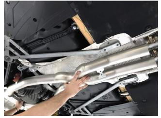
**Step 16:** With the forward midpipe in place, install the gray hangers and bracket in place securing with the previously removed torx bolts.
