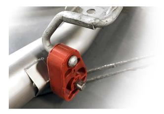
**Step 13a:** Install the previously removed orange hangers onto the Soul Performance Products exhaust
