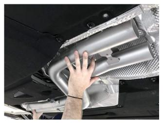
**Step 13b**: Install the previously removed orange hangers onto the Soul Performance Products exhaust
