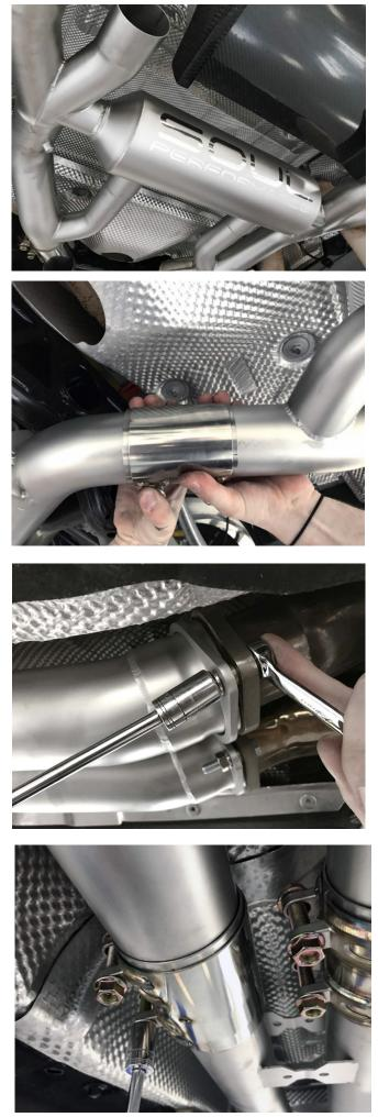
**Step 24**: With the black hangers and brackets already installed, lift the muffler section into place and secure the hanger bracket with the previously removed 15mm nuts (Step 7)
