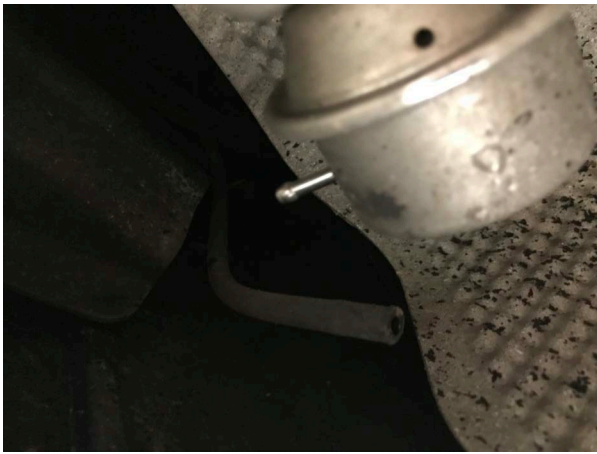
Pictured Left: Unbolt the factory exhaust hangers to release the factory rear mufflers from the car.
