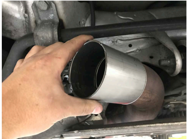
Pictured Left: Transfer the OEM exhaust hangers over to your Soul Performance exhaust.
