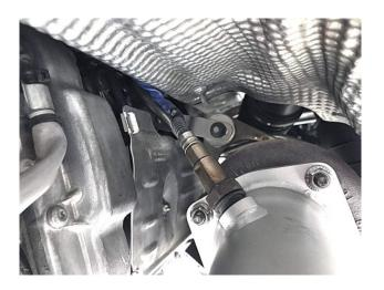
**Step 17:** Install the secondary O2 sensor. Torque to 37 - 44 ft-lb.
