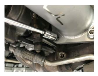
**Step 13:** Using the included 13mm locking nuts and washers loosely install the first Sport Cat section to the turbo to allow the system to sag making o2 sensor installation easier.
