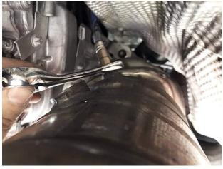
**Step 7:** Remove both primary O2 sensors (22mm).
