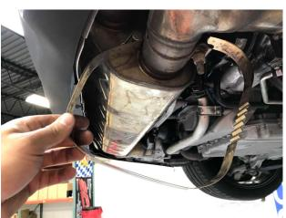
**Step 2:** Locate and **VERY CAREFULLY** remove the EGT sensors (14mm). If they bend or twist you will damage the ceramic in the sensor.
