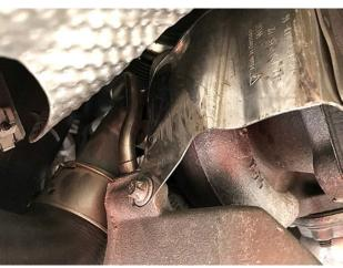
**Step 8:** Remove the final 8mm nuts holding the turbo heat shields on.
