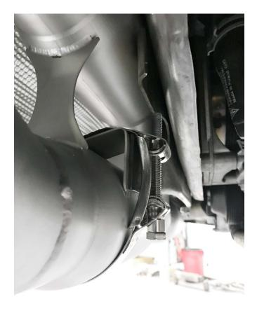
**Step 23:** Once both sides of the Sport Cat sections are loosely installed, fully tighten down the 2.5" Accuseals.
