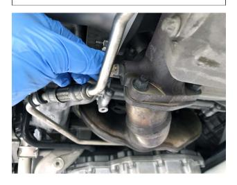
**Step 16:** Install the primary O2 sensor first. Torque to 37 - 44 ft-lb.
