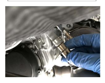
**Step 18:** Make sure the O2 sensor harness is back on the clip.
