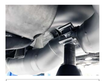
**Step 24**: Once positioned correctly fully tighten the custom Mikalor clamps that were provided.
