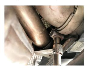
**Step 1:** With the car supported safely, locate and loosen the bolt clamp (E12mm) holding the exhaust tips, then remove the tips from the vehicle.
