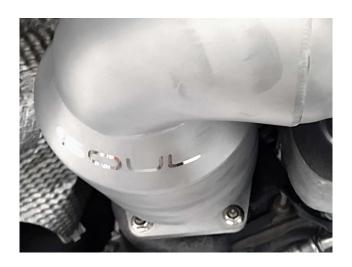
**Step 20:** Slip on the provided 2.5" Accuseals onto the X-Pipe section.
