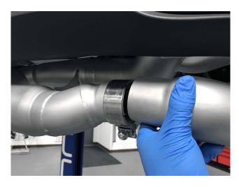
**Step 22:** Use both of the provided Mikalor clamps to position and hold the X-Pipe against the OEM bracket. Lightly tighten the clamps.
