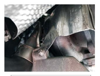
**Step 15:** CAREFULLY hand screw in the EGT sensor then carefully tighten it down.
