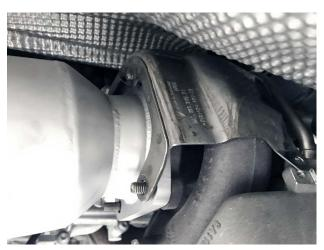
**Step 12:** Place the OEM turbo heat shield in the correct location.
