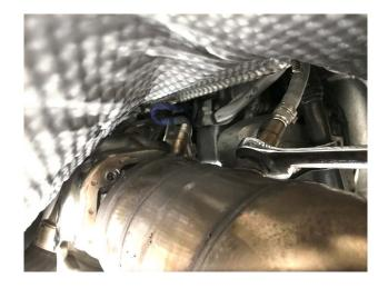
Step 6: Remove Secondary O2 Sensors (22mm).
