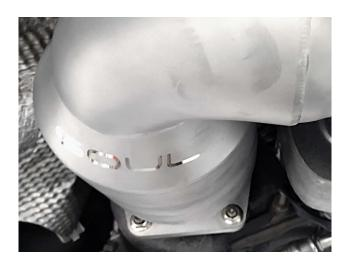
**Step 22:** With all sensors now installed, fully tighten and torque the included 13mm locking nuts and washers on the turbos.
