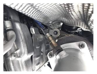
**Step 18:** Install the Primary O2 Sensors first.
