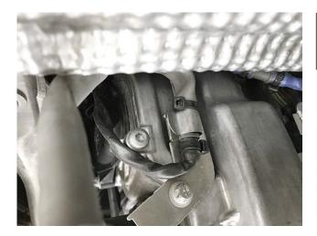
**Step 21:** Loop the the OEM band clamp back around the OEM muffler.
