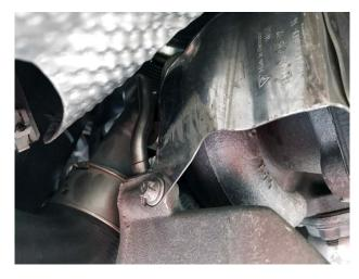
**Step 16:** Install 8mm turbo heat shield bolt back onto shield.
