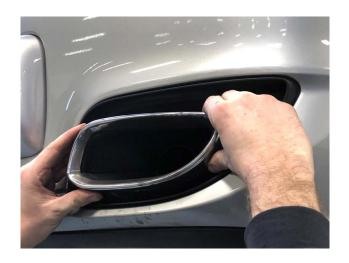
**Step 25:** Slip on and adjust the tips onto the OEM muffler to your desired position. Tighten down the clamps for the tips.
