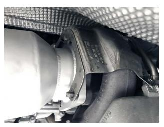
**Step 14:** Place the OEM turbo heat shield in the correct location.
