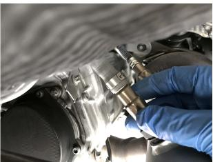
**Step 19:** Install the Secondary O2 Sensors.
