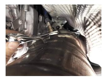
**Step 7:** Remove both Primary O2 sensors (22mm.
