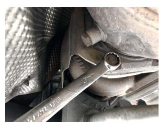
**Step 4:** Loosen and remove the nuts holding the exhaust to the turbochargers. (4 13mm nuts on each side)
