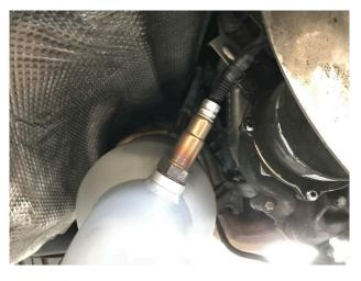
**Step 15:** Reinstall and tighten the O2 sensors.
