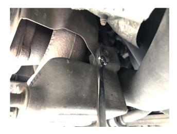
**Step 5:** Loosen and remove turbocharger heat shields.
