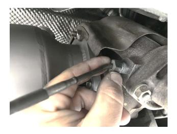
**Step 13:** Reinstall EGT sensors on both turbos and torque them down.
