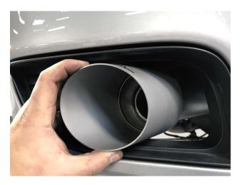
**Step 20:** Install and adjust exhaust tips with 13mm socket wrench.
