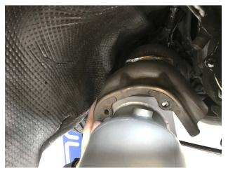
**Step 11:** Position heat shield over the turbo flange and install new Sport Cat sections.
