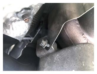
**Step 14:** Reinstall heat shield bolts and tighten.
