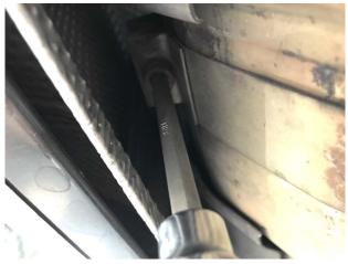
**Step 6:** Unbolt both OEM muffler band straps while supporting the muffler using M6 allen socket / extension.
