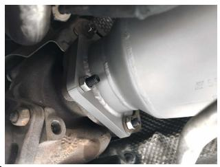
**Step 12:** Install new included nuts and washers and torque down on both sides.
