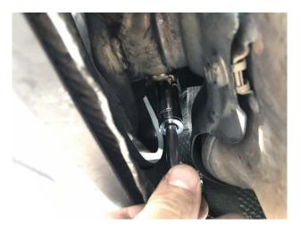
**Step 2:** Loosen and remove both OEM exhaust tips (13mm bolts).
