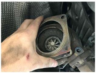
**Step 10:** Clean and reinstall OEM turbo gaskets if in good condition, or install new OEM gaskets.
