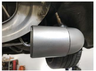
**Step 16:** Slide exhaust couplers onto each exhaust end.
