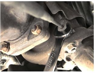
**Step 3:** Remove the EGT sensors on each turbo using a 14mm wrench.
