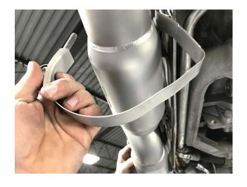
**Step 17:** Install x-pipe and exhaust hanger clamps. Use the exhaust couplers to support the x-pipe while you do this to make the installation easier. Tighten the exhaust straps.
