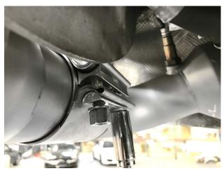
**Step 18:** Tighten the exhaust couplers to seal the system.
