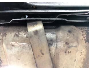
**Step 8:** Slide muffler straps off the muffler bracket.
