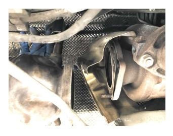
**Step 9:** Adjust turbo heat shield to be able to remove the exhaust down and out of the vehicle.
