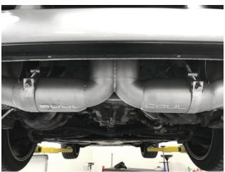
**Step 15:** Center X-pipe section into alignment and tighten band clamps.
