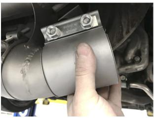
**Step 18:** Slide Torca clamps onto tip outlets.
