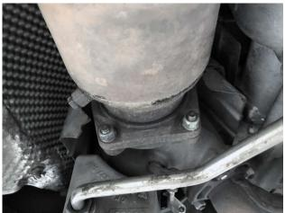
**Step 2:** Loosen and remove the nuts holding the exhaust to the turbochargers. (Four 13mm nuts on each side)
