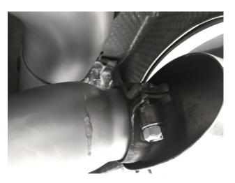
**Step 20** Install tip outlet pipes
