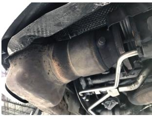
**Step 8:** Pull factory exhaust free from turbo studs and carefully remove from vehicle.
