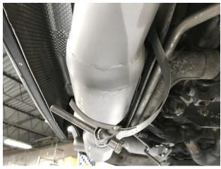
Step 14: Install new band clamps loosely
