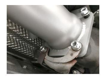
**Step 17:** Tighten and fully torque down exhaust to turbo bolts and heat shield bolts.
