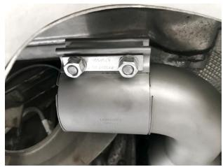
**Step 12:** Slide Torca clamps onto ends of catless pipes.
