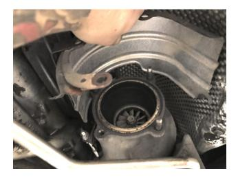
**Step 9:** After removing exhaust, put heat shields back in place
