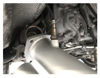
**Step 11:** LOOSELY install catted sections and install O2 sensors (catless pipes pictures). This allows for play later when installing center X-pipe section.
