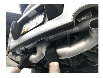
**Step 13:** Install X-pipe section by lining up with catless sections and slide Torca clamps over.
