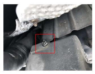
**Step 3:** Remove turbo heat shield bolt on both turbos.
