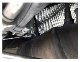
**Step 7: CAREFULLY** lower exhaust slightly then remove all four O2 sensors (22mm wrench).
