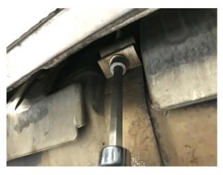
**Step 5:** Unbolt both OEM muffler band straps while supporting the muffler using M6 allen socket / extension.
