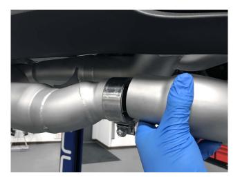
**Step 22:** Use both of the provided Mikalor clamps to position and hold the Sport Cats against the OEM bracket. Lightly tighten the clamps.
