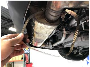
**Step 2:** Locate and **VERY CAREFULLY** remove the EGT sensors (14mm). If they bend or twist you will damage the ceramic in the sensor.
