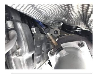
**Step 17:** Install the secondary O2 sensor.
