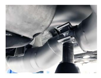
**Step 24**: Tilt the top part of the center X-pipe slightly forward to align the tip outlets with the bumper. Once positioned correctly fully tighten the custom Mikalor clamps that were provided.
