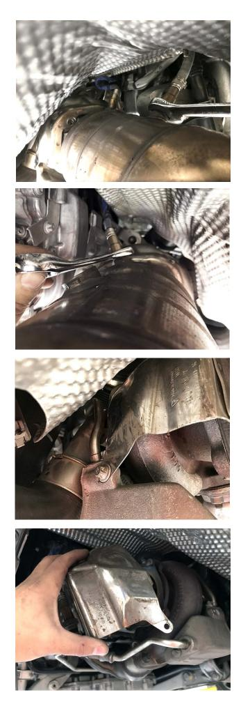
**Step 6:** Remove secondary O2 Sensors (22mm).
