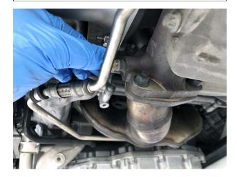
Step 16: Install the primary O2 sensor first.
