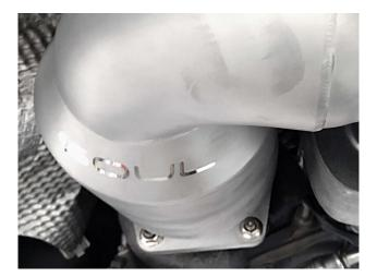
**Step 20:** Slip on the provided 2.5" Accuseals onto the X-Pipe.
