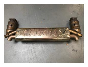
**Step 9: At this time remove the final nuts holding the system onto the car, and** remove the heat shields and OEM exhaust system from the vehicle. You will most likely have to use some force to remove it. Mind the space between the exhaust and bumper to prevent any possible damage.
