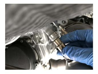
**Step 18:** Make sure the O2 sensor harness is back on the clip.
