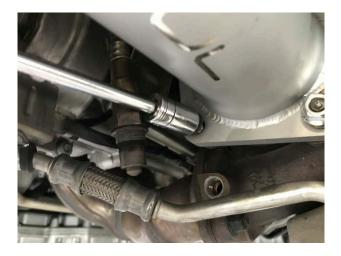
**Step 13:** Using the included 13mm locking nuts and washers loosely install the first Sport Cat section to the turbo to allow the system to sag making o2 sensor installation easier.
