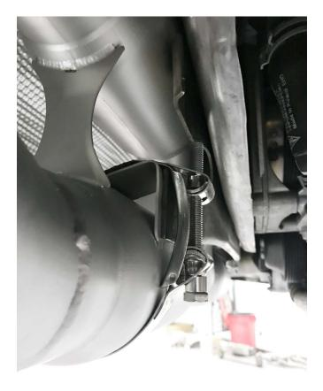
**Step 23:** Once both sides of the Sport Cats are loosely installed, fully tighten down the 2.5" Accuseals.
