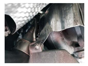
**Step 15:** CAREFULLY hand screw in the EGT sensor then carefully tighten it down.
