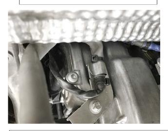
**Step 19:** With all sensors now installed, torque down the included 13mm locking nuts and washers on the turbos.
