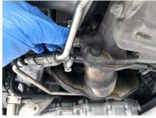
**Step 17:** CAREFULLY hand screw in the EGT sensors then carefully tighten them down.
