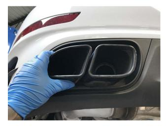
**Step 25:** Slip on and adjust the tips onto the OEM muffler to your desired position.
