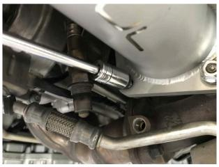
**Step 15:** Using the included 13mm locking nuts and washers loosely install the Cat Bypass Pipes to the turbo to allow the system to sag making o2 sensor installation easier.
