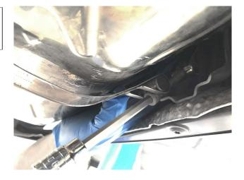
**Step 24:** Tighten down the OEM clamps holding the Cat Bypass Pipes to the muffler to 41 ft/lbs.
