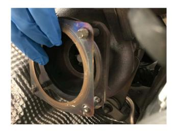
**Step 12:** You may replace or reuse the OEM turbo gaskets if they are in good condition.
