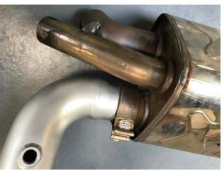
**Step 11:** Install the Soul Performance 991 Turbo Sport Catalytic Converters **tight but NOT fully torqued** - you will need to adjust once the exhaust assembly is installed back on the vehicle.
