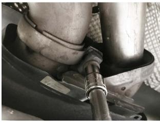
**Step 26:** Finally tighten down the clamps for the tips once they are in your desired position.
