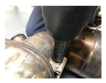
**Step 10:** Locate the OEM clamps holding the OEM catalytic converters. Loosen the clamp bolts with a 15mm socket and remove the OEM catalytic converters.
