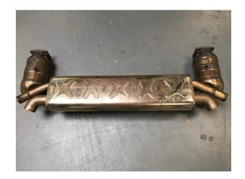
**Step 9: At this time remove the final nuts holding the system onto the car, and** remove the heat shields and OEM exhaust system from the vehicle. You will most likely have to use some force to remove it. Mind the space between the exhaust and bumper to prevent any possible damage.
