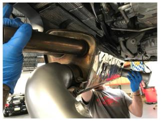
**Step 13:** Lift the OEM muffler with Sport Catalytic Converters installed and position the muffler in place while orienting the converters into the correct location for installation.
