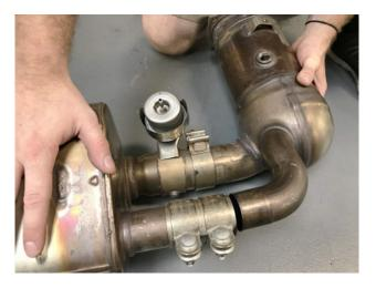
**Step 9:** Using a 15mm socket, loosen the accuseal clamp on the larger pipe and 13mm socket to loosen the torca clamp and slide the catalytic converter out.
