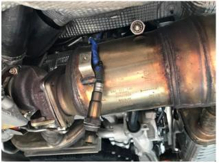
**Step 4b:** With both oxygen sensors removed you can tuck them out of the way.
