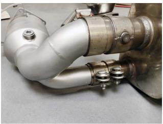
**Step 10:** Install the Soul Performance Products Sport Catalytic Converters into position, leave assembly loose to allow for adjustments later.
