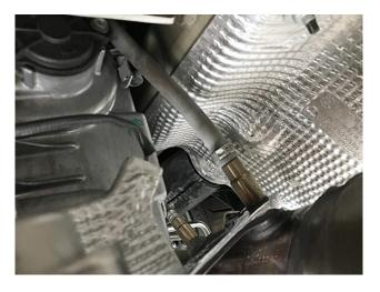
**Step 4:** Using a 22mm wrench loosen and remove both oxygen sensors. Be mindful of their positions (primary and secondary locations) and mark them if necessary to ensure that you re-install them in the correct position.
