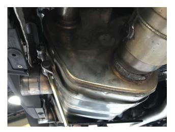
**Step 13:** Install the band straps over the center muffler and muffler mounting bracket and tighten the 6mm allen head.
