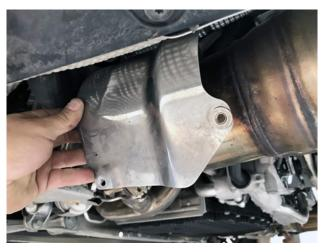
**Step 2:** Carefully remove the heat shield and keep the hardware close, you will be reinstalling it later in the guide.
