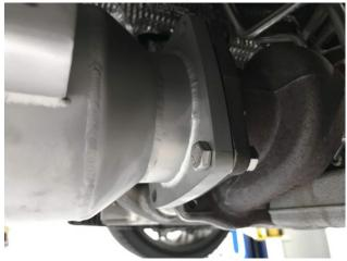
**Step 12**: Guide the exhaust and catalytic converters up and into position and tighten the hardware with the 4 nuts and 3 bolts provided. One nut will be placed on the factory stud on the turbo.
