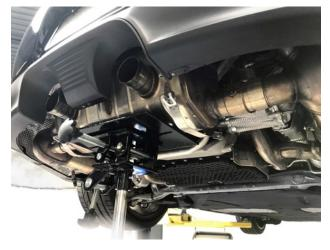
**Step 7:** Support the muffler with the help of a friend or a transmission jack.
