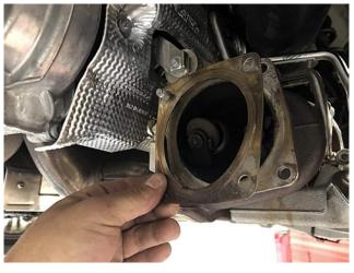
**Step 11**: Clean the flange on the turbo of any debris and reinstall the OEM metal gasket. You can use a copper gasket sealant to aid in this process.
