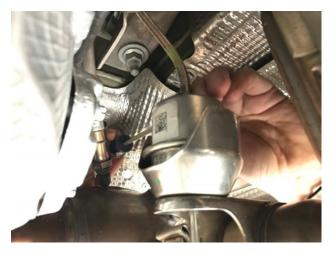
**Step 5:** Remove the vacuum hose to the factory PSE valves.
