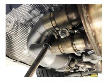
**Step 14:** Tighten the accuseal and torca clamp locking the center muffler and catalytic converters together.
