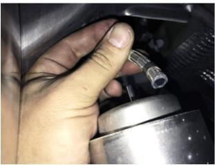
**Step 17**: Reinstall the factory vacuum hoses to the two valves on the PSE muffler.
