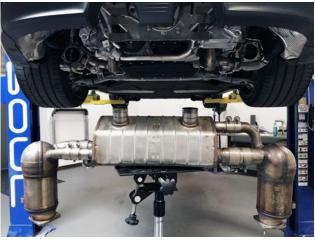
**Step 8:** Carefully slide the exhaust towards the rear of the car and gently lower it out being careful not to damage the studs on the turbo.
