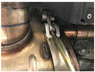
**Step 6:** Moving to the center muffler, using a 6mm allen drive loosen the band strap and slide it to the outside of the muffler.
