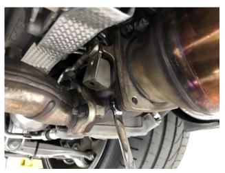
**Step 3:** Using a 12mm wrench, loosen and remove the hardware holding the catalytic converter to the turbo. Be careful to not damage the one stud on the turbo side, you will be re-using it.
