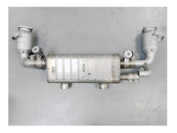
**Pictured Left:** Exhaust system loosely assembled and ready for reinstallation.
