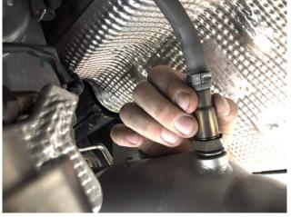
**Step 15:** Reinstall the oxygen sensors using anti seize and a 22mm wrench.
