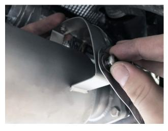
**Step 16:** Reinstall the factory heat shields onto your Soul Performance Products Sport Catalytic Converters.
