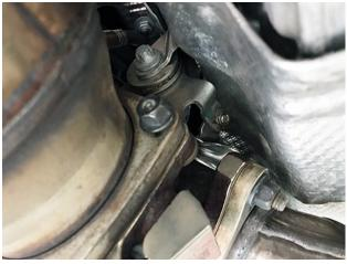
**Step 1b:** The two torx bolts on the turbo can be tough to see. There is one on the left and one on the right side of the turbo.
