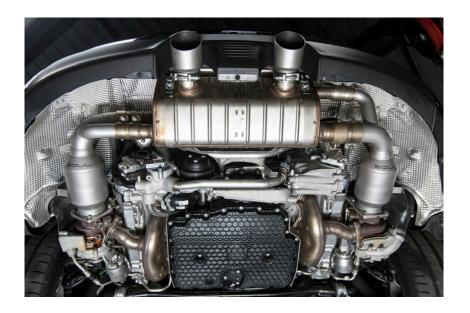
**Pictured Left:** Newly installed Soul Performance Products Sport Catalytic Converters.
