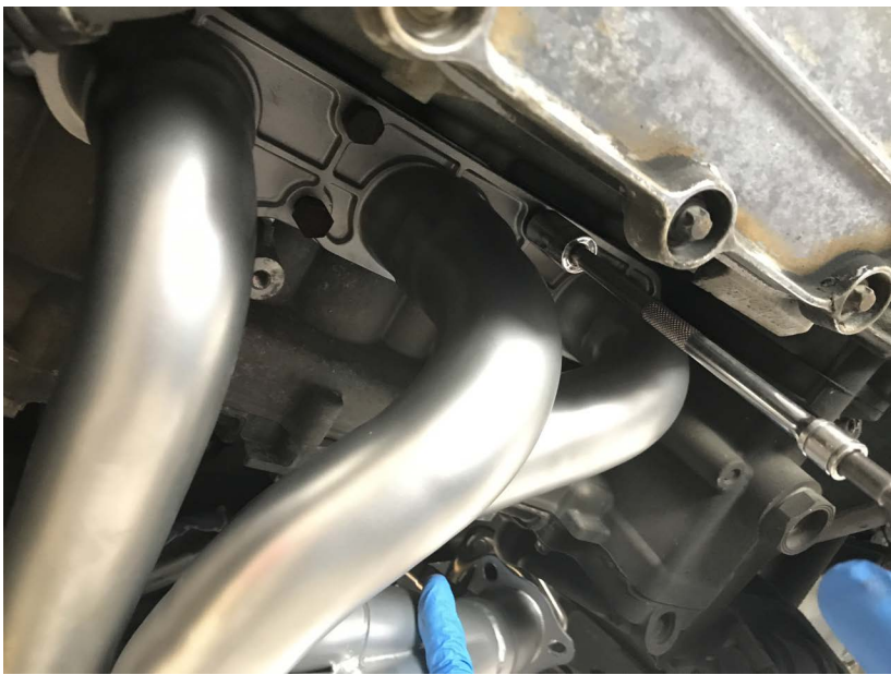
Pictured Left: Install the factory 13mm bolts into position and torque to factory specification. ***Tip: Start from the inner most bolts and tighten outwards following an alternating path side to side
