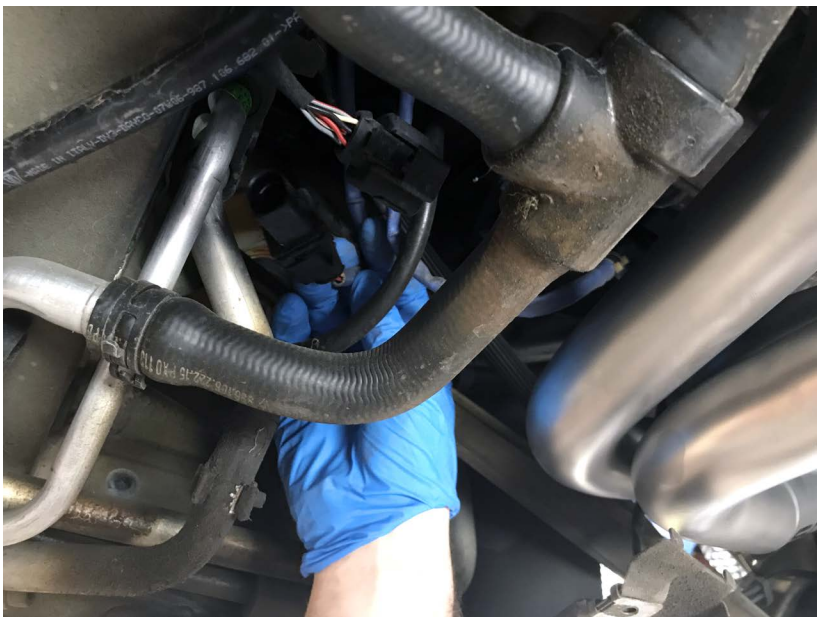
Pictured Left: Re-route your oxygen sensor wiring and tie downs in the reverse sequence of removal
