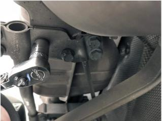
Remove factory hardware from the rear mounting bracket. (two) 13mm nut & bolt combinations per side.
