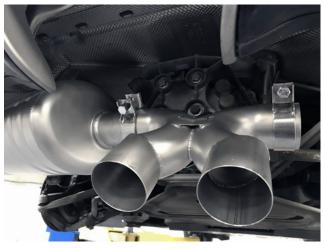
Install and loosely tighten the SOUL exhaust outlet "X" Pipe.
