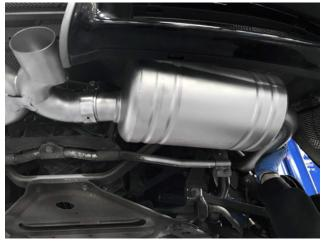
With the 3 bolt gasket coated and in place, install the passenger side portion of you SOUL exhaust into position and insert the outlet pip on the muffler into the outlet "X" Pipe.
