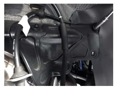
Start by raising your car and removing the rear wheels. Then remove the tire shield from the fender wells (three 10mm bolts and four T-25 Torx bolts) on both sides (it is not absolutely necessary to remove the wheels and tire covers, it will however make the install much easier.
