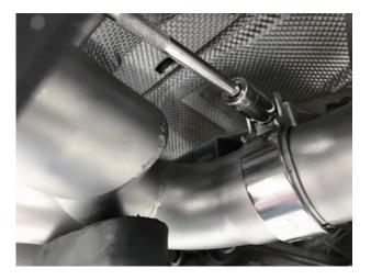
After positioning the outlet "X" pipe height as desired, remove the SOUL exhaust tips to allow enough room to tighten the 13mm hardware on the outlet "X" pipe locking it in place.
