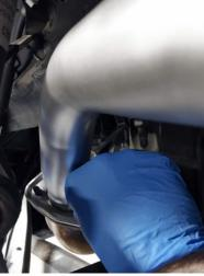
Slide the driver's side half of your new Soul Performance Exhaust up and into its position. Loosely tighten the three 13mm supplied nuts onto the header flanges enough to provide support but still loose enough to allow for adjustment later.
