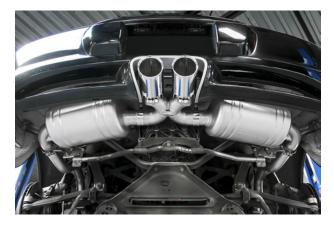
Reinstall the Soul Performance exhaust tips and set the depth as desired. Tighten the 10mm bolts on the clamps.
