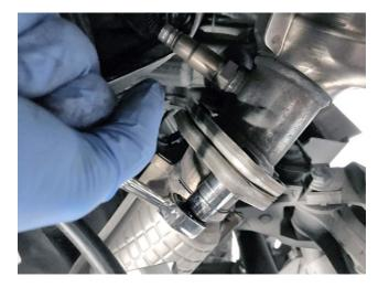
Remove factory mounting hardware from the header/muffler flanges on both sides. In most applications these will be a 13mm nut/bolt combination.
