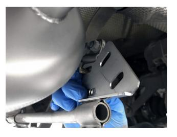
Install the supplied inner half of the SOUL exhaust support bracket loosely with the two 13mm nut/bolts.
