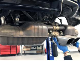
You can now slide the exhaust rear and downwards to remove it from the car.
