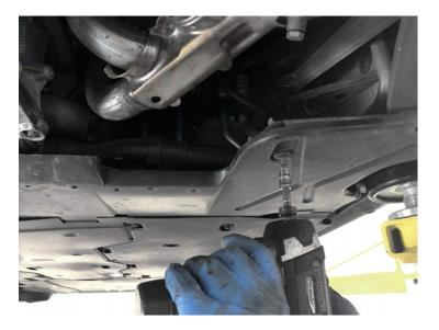
**Pictured Right:** Remove the three 13mm nuts at the header to muffler flange on both sides.
