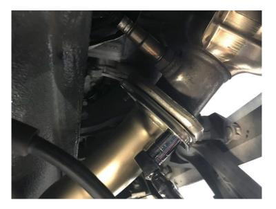
**Pictured Left:** Locate the oxygen sensor wiring mounting locations and disconnect / remove the sensor clips and tie downs.
