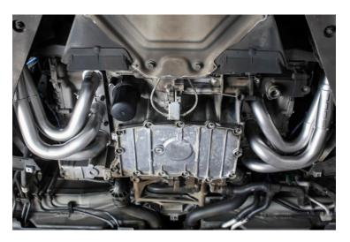
**Pictured Left:** Ensure that all hardware is tightened and any electrical wiring is properly secured and out of the way. Then install any panels you have removed
