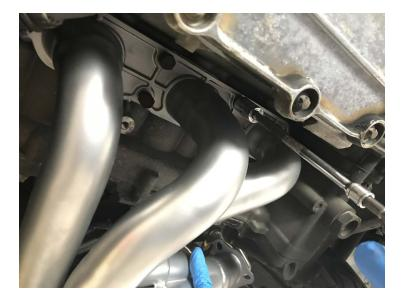
**Pictured Left:** Install the factory 13mm bolts into position and torque in the factory sequence shown below. **Factory specs call for 23 Nm / 17 ft-lbs of torque.** Less may result in the hardware coming loose and more may result in stripped or broken hardware in the aluminum head - tighten with care!
