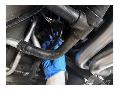
**Pictured Right:** Install the supplied header flange to muffler flange gaskets and torque to factory specifications. It is okay to re-use your factory gaskets if they are in good condition and you have applied a coat of copper gasket sealant. If you plan on tracking the car frequently, we recommend using OEM Porsche gaskets.
