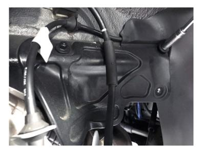
**Pictured Left:** Start by raising your car and removing the rear wheels. Then remove the tire shield from the fender wells (two 10mm bolts and one T-25 Torx bolts) on both sides (it is not absolutely necessary to remove the wheels and tire covers, it will however make the install much easier.)
