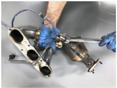
**Pictured Left:** Coat the oxygen sensors with an antiseize of your choice
