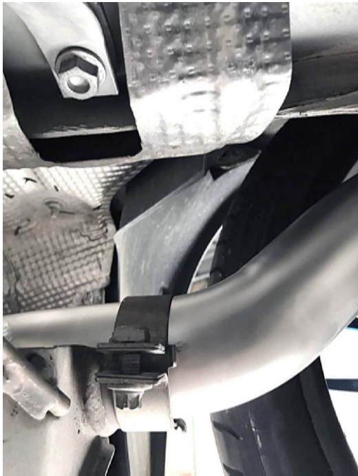
Pictured Left: Install the passenger’s side SOUL muffler following the same procedure as the previous side. Slide the muffler outlet into the outlet “X” pipe and loosely tighten. At this point you can start to tighten all exhaust hardware to torque except the outlet “X” pipe . Start from the front of the exhaust and work rearwards tightening each side equally alternating between them.
