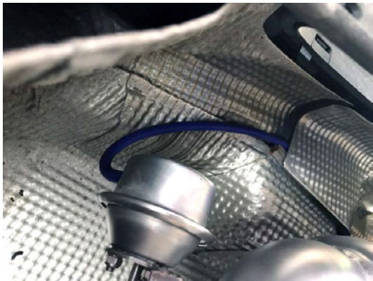
Pictured Left / Below: Install the supplied vacuum hose and route out of the way either as photographed or to your liking. Connect each side to their respective valves, one on the driver's side and one on the passenger's side of the exhaust.
