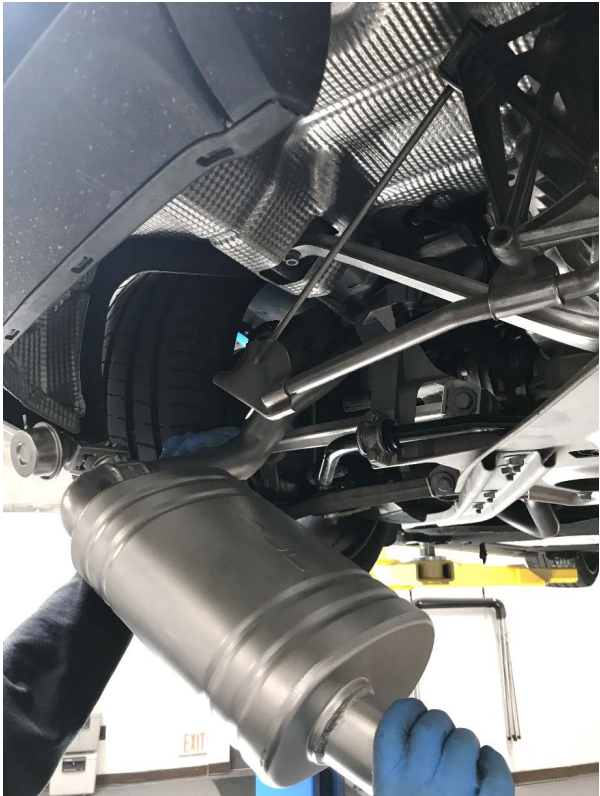
Pictured Left: If your factory gaskets are in good shape it is okay to coat them in a copper gasket sealant and re-use them. If you plan on racing the vehicle, OEM Porsche gaskets are recommended. Otherwise, install the supplied gasket. Loosely install the two supplied nuts/bolts (13mm) into the header/muffler flange. Leave them loose enough to allow for adjustment later.
