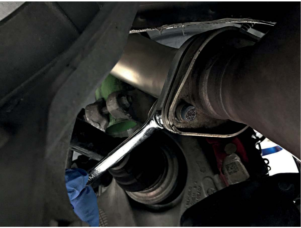
Pictured Left: Remove the 13mm bolts securing the header/muffler flange bolts (2 per side). You will not be re-using these.
