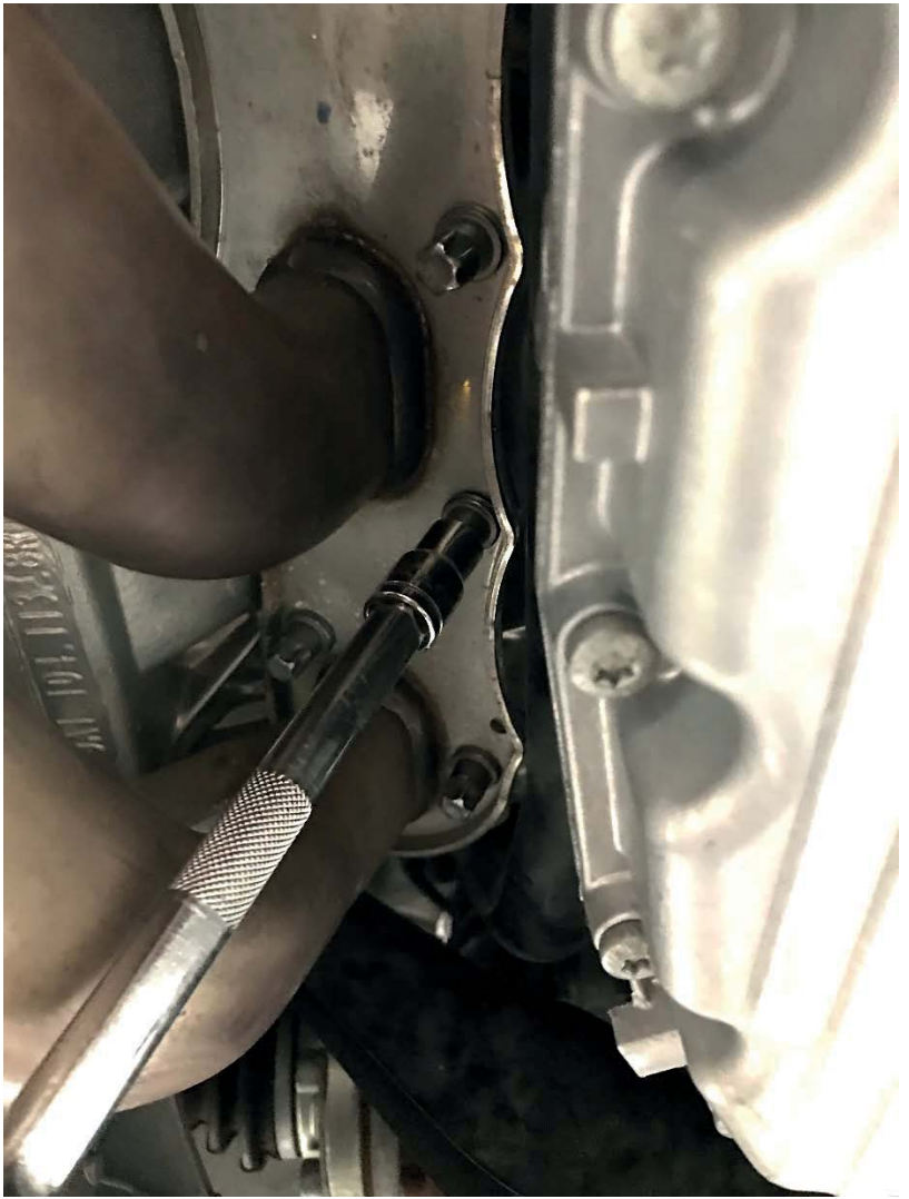
Pictured Left: Remove the E-12 Torx bolts from the header flanges. There are 9 per side, you will be re-using these.
