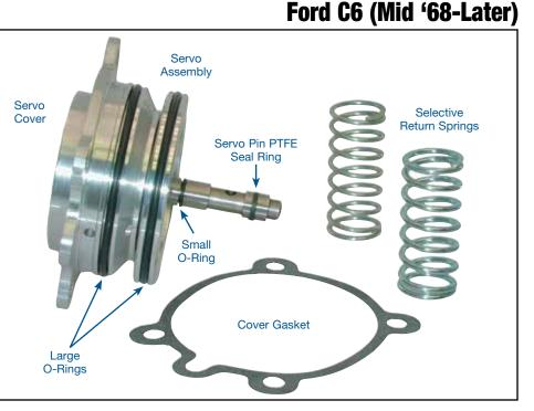
a. This servo kit is a drop-in item for mid '68-later models. Models previous to this will need to be bored out to 3.493"/3.495" dia. with a surface finish of less than RA16.
