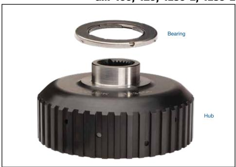
**WARNING:** Compared to OE or other replacement forward clutch hubs, this hub and bearing combination has an additional .025" thickness designed-in to reduce endplay and provide further endplay adjustment options.
