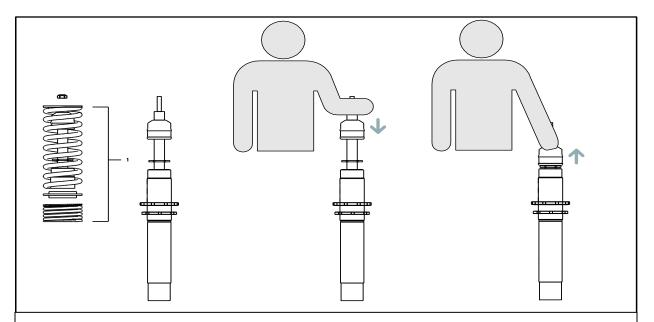
SOLO WERKS TIP: As the suspension is shipped and stored in a horizontal position, it is advisable to exercise or Prime the shock absorber before you install them to ensure that the internal contents are in the correct chambers. Therefore, we advise that before you assemble the front coilover shock absorber, take a moment to purge the shock absorber.
