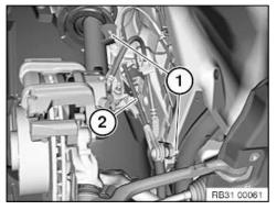
6. Remove Lower spindle (Pinch) Bolt from spindle (1&3)
