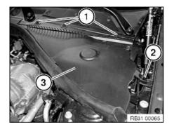
3. Remove three (3) upper strut mount bolts and the 1x strut tower brace bolt
