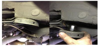
5. Remove the upper bolts from the upper shock mount on each side & remove rear shocks.
