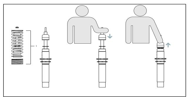
SOLO WERKS TIP: As the suspension is shipped and stored in a horizontal position, it is advisable to exercise or Prime ALL shock absorbers before you install them to ensure that the internal contents are in the correct chambers. Therefore we advise that before you assemble the front coilover shock absorber, take a moment to purge the shock absorber.
