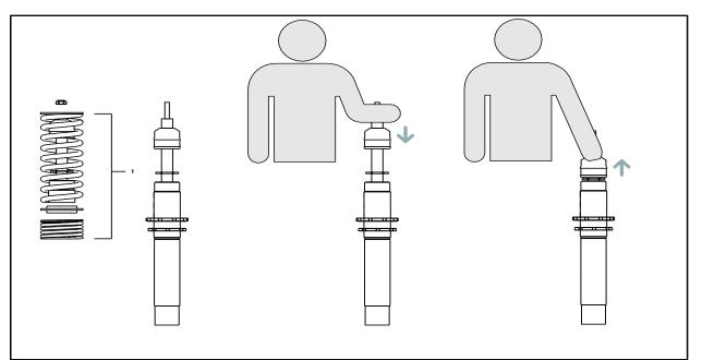
SOLO WERKS TIP: As the suspension is shipped and stored in a horizontal position, it is advisable to exercise or Prime the shock absorber before you install them to ensure that the internal contents are in the correct chambers. Therefore we advise that before you assemble the front coilover shock absorber, take a moment to purge the shock absorber.
