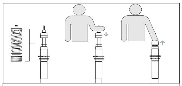
SOLO WERKS TIP: As the suspension is shipped and stored in a horizontal position, it is advisable to exercise or Prime the shock absorber before you install them to ensure that the internal contents are in the correct chambers. Therefore, we advise that before you assemble the front coilover shock absorber, take a moment to purge the shock absorber.
