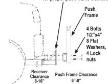
bolt pattern is too high, remove interceptor and turn leg down. Bolt push frame (4 bolts 1/2" x 4" w/ flat washers and lock nuts) to proper hole height on interceptor – leave bolts snug tight for now.
