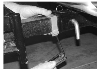
b) Push set collar tight against receiver – hold and tighten set screw with 3/16" allen wrench.
