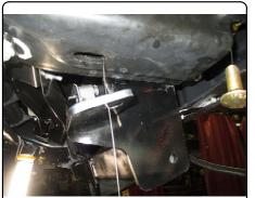
5. Secure all hardware and torque all 1/2" hardware to 110 ft-lbs and all M12-1.75 to 86 ft-lbs. Reconnect electrical harness through hole in driver side plate.
