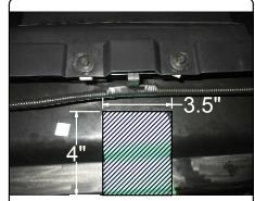
4. Raise side plates into position and loosely secure (4) hex flange nuts onto existing bolt plates or 1/2-13 x 1 1/2" bolts. Fishwire supplied (2) 1/2-13 x 1 1/2" carriage bolts and CM-SP10 spacers through front of driver and passenger side frame rails and out slot on bottom of frame rail. Loosely secure 1/2-13 hex flange nuts onto carriage bolts.
