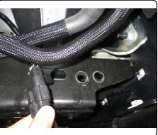
2. Fishwire (2) bolt plates removed in STEP 1 through original holes on inside of frame rails.
