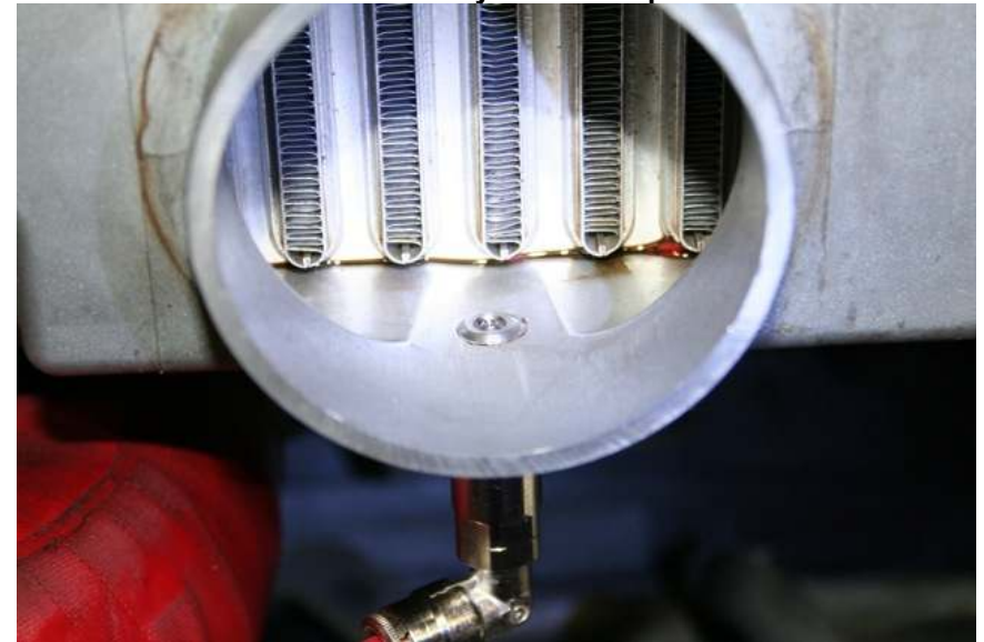
Nozzle mounted at the outlet of the factory intercooler. Note the slight projection of the nozzle tip into the airflow.
