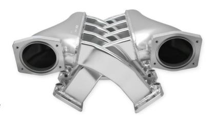
four cylinders and the tapered shape of the plenum help increased air velocity directed to each of the intake runner ports.
