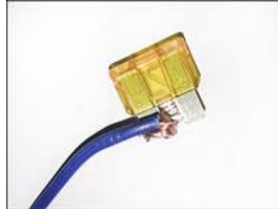
Wire Jammed Into a Fuse
