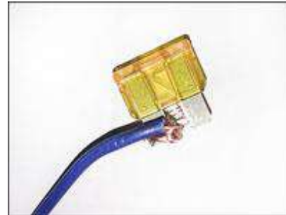
Wire Jammed Into a Fuse
