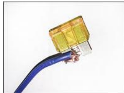
Wire Jammed Into a Fuse
