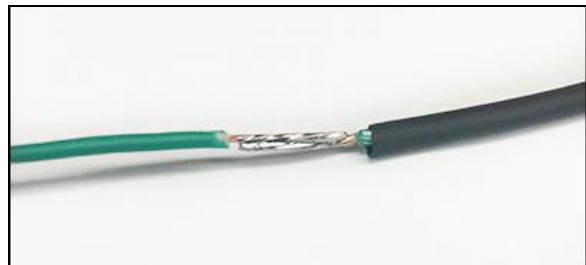
Soldered Connection w/ adhesive heat shrink
