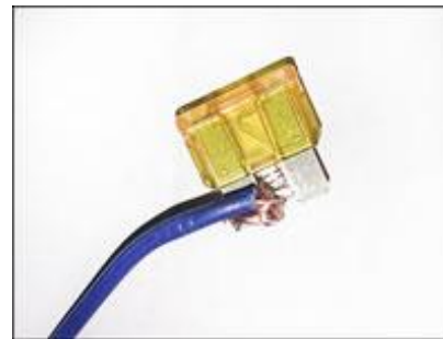
Wire Jammed Into a Fuse
