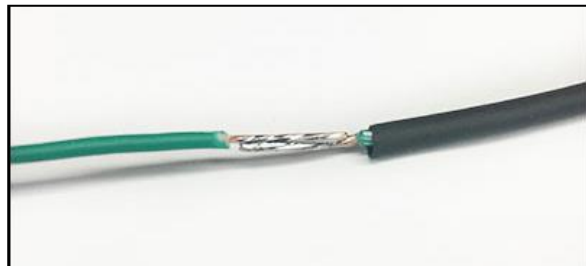
Soldered Connection w/ adhesive heat shrink
