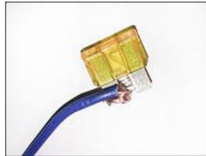
Wire Jammed Into a Fuse
