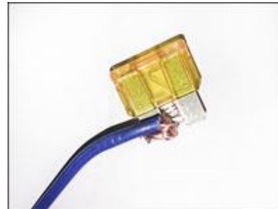
Wire Jammed Into a Fuse
