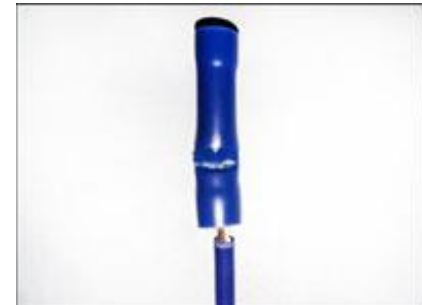
Broken Butt Connectors
