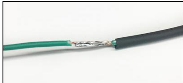
Soldered Connection w/ adhesive heat shrink
