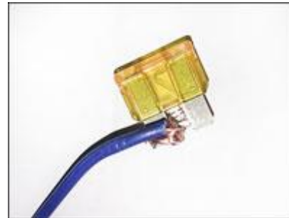
Wire Jammed Into a Fuse
