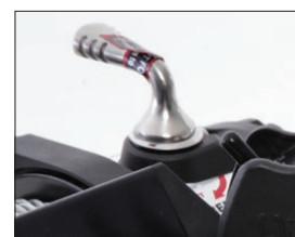
LARGER CLUTCH LEVER FOR EASE OF USE WITH GLOVES
