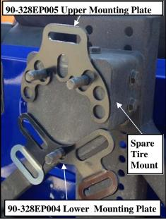
$\underline{\text{Step 3:}}$  Install the (3) nylon strap (90-328EP008) hooks into the upper (90-328EP005) and lower (90-328EP004) mounting plates. (Fig. A)
