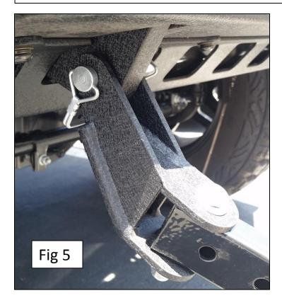
Step 7. Center tow bar and brackets on vehicle, then tighten all hardware. Check torque on all hardware and inspect tow bar before each used.
