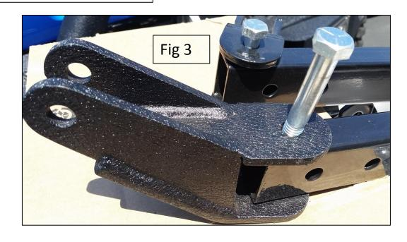
Step 5. Insert shackle spacer into shackle mount on bumper. Play is normal, if you wish you may use some tape on spacer to help it stay in place during the install of the tow bar. Fig 4
