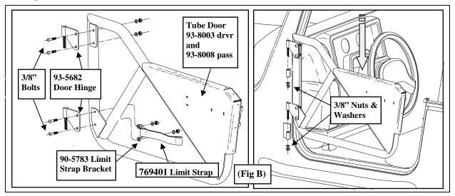
**<u>Step 6:</u>** Carefully install the door assembly onto the vehicle hinges. (Fig B)
