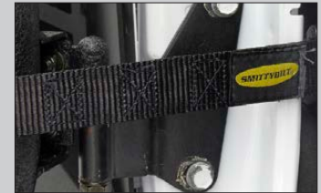
D Door straps included. Mounts to factory hinges
