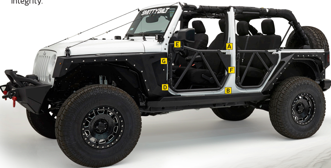
D Door straps included. Mounts to factory hinges
