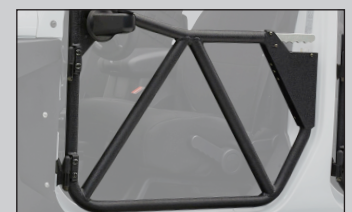
G 1.75" diameter 0.120 wall steel tubing
