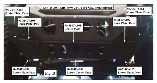
Step 10: NOTE: This step might require 2 people. Raise the new front bumper (93-312CA002 SRC or 93-314DV002 XRC) up into place and align the bumper mounting studs with (4) holes on the frame mounting plates. Secure using the previously removed OE hardware. (Fig D)
