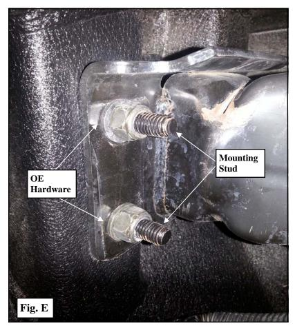
**Step 11:** Level the bumper and torque the **OE** hardware to manufacturer's specifications. (Fig E)
