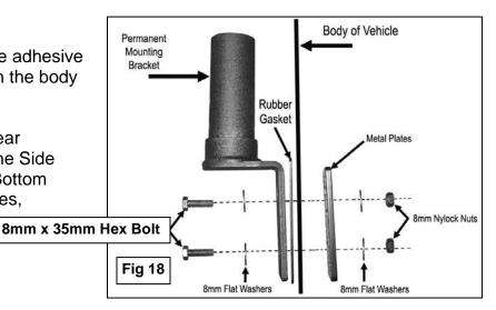
**24.** Insert (2) 8mm x 35mm Hex Head Bolts with (2) 8mm Flat Washers through the Short Bottom Brackets and body. Access the hardware through the opening for the taillight and position the 2-hole Metal Plates over the already inserted 8mm Hex Bolts, **(Figure 19)**.
