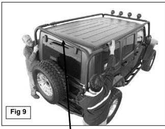
IMPORTANT! Do not lay Roof Rack on your vehicle to attach the Rear Bottom Legs at any time. Damage to the vehicle may occur.
