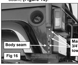
Mark location to drill 3/4" from seam-toward rear of vehicle
