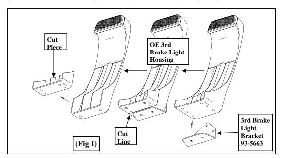
**Step 3:** Once the **OE** 3rd brake light plastic housing has been properly trimmed, place it flush against the back 3rd brake light bracket (**93-5663**). Use the **(3)** holes in the bracket as a
