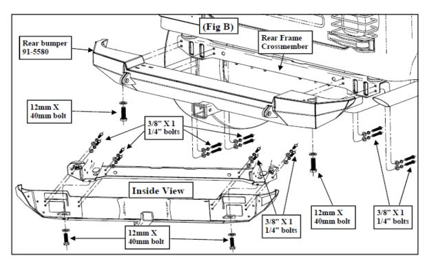
Step 5: Install the (4) 3/8" X 1 1/4" bolts and hardware into the previously drilled inner mounting holes in the rear frame crossmember. (Fig B)
