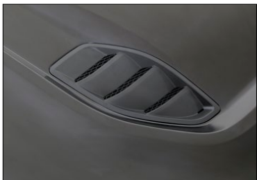
Vent hot gases out of engine bay
