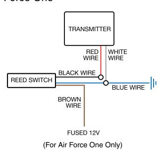
Connect the red wire on the Wireless CoachLink Transmitter to the black wire on the reed switch.
