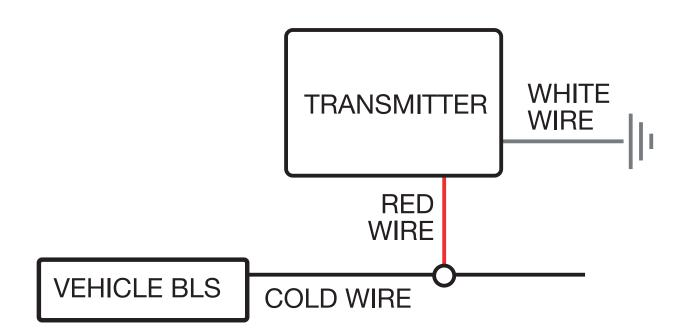
Note: If the vehicle has an inactive brake light switch, meaning the cold wire does not receive voltage when the key is in the tow position an add-on brake light switch will need to be installed separately.
