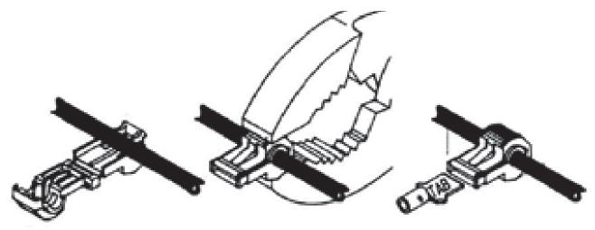
Using Pliers clip the red flipover spade connector over the cold side of the brake light switch. If your vehicle has an inactive brake light switch connect the red flipover spade connector to the cold side of the aftermarket brake light switch.
