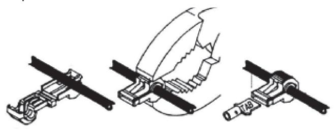
Using Pliers clip the red flipover spade connector over the cold side of the brake light switch. If your vehicle has an inactive brake light switch connect the red to the blue wire of the Stay N Play DUO operating unit that is under the hood of the towed vehicle.
