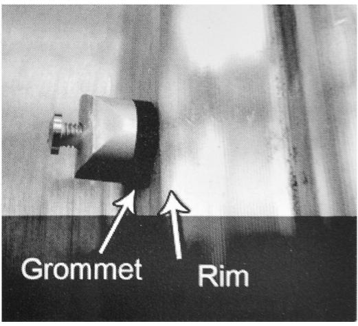
B) With one hand adjust the angle of the sensor according to the contour of the wheel and hold in place. Use a Philips head screwdriver to tighten the screw (1) on the back of the valve stem. Securely fasten the valve/sensor assembly to the wheel by tightening the 11 mm nut to 35 in-lbs (4 N-m) using an in-lbs torque wrench.
